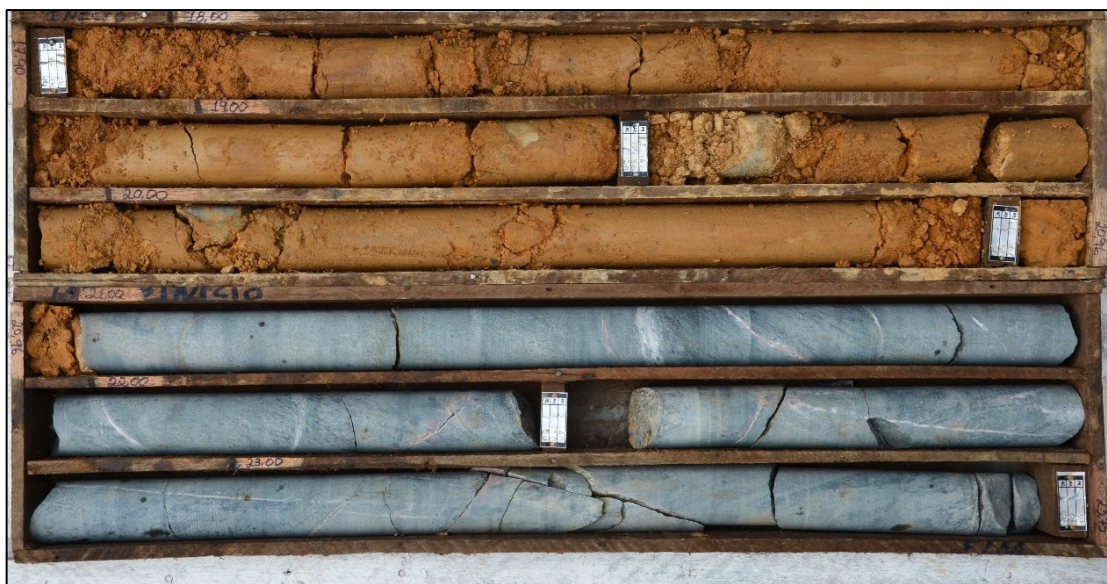
Figure 16-14: Sharp contact between saprolite and fresh rock (Borehole 19-027: 17.90 m to 23.75 m)
