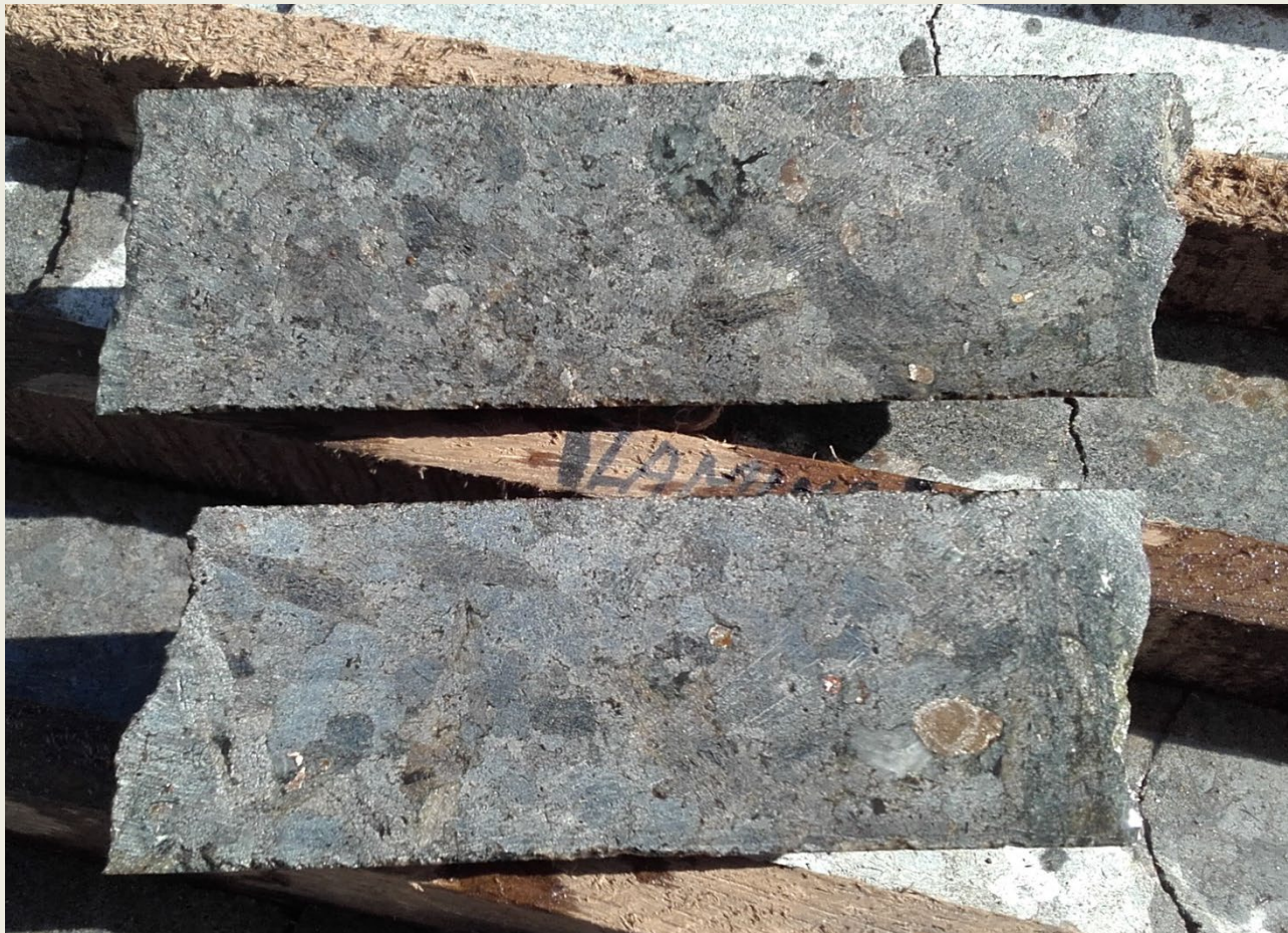
Peridotite with rounded blebs of sulphide
