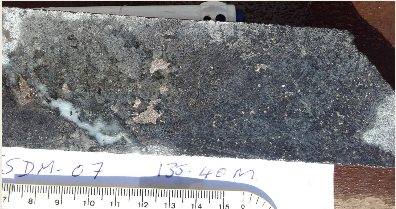
Hole FSDM-07. Peridotite with coarse sulphide aggregates from 135.4m
