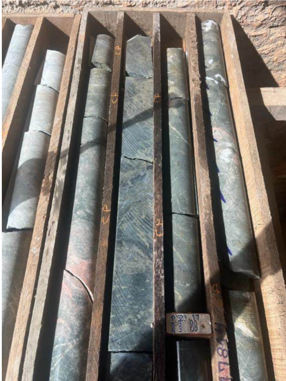
Figure 10-9: Photograph of very competent section of core in a chalcopyrite mineralized section of porphyritic andesite core with pinkish K-Feldspar-epidote veining and visible chalcopyrite mineralization (cp markings).
