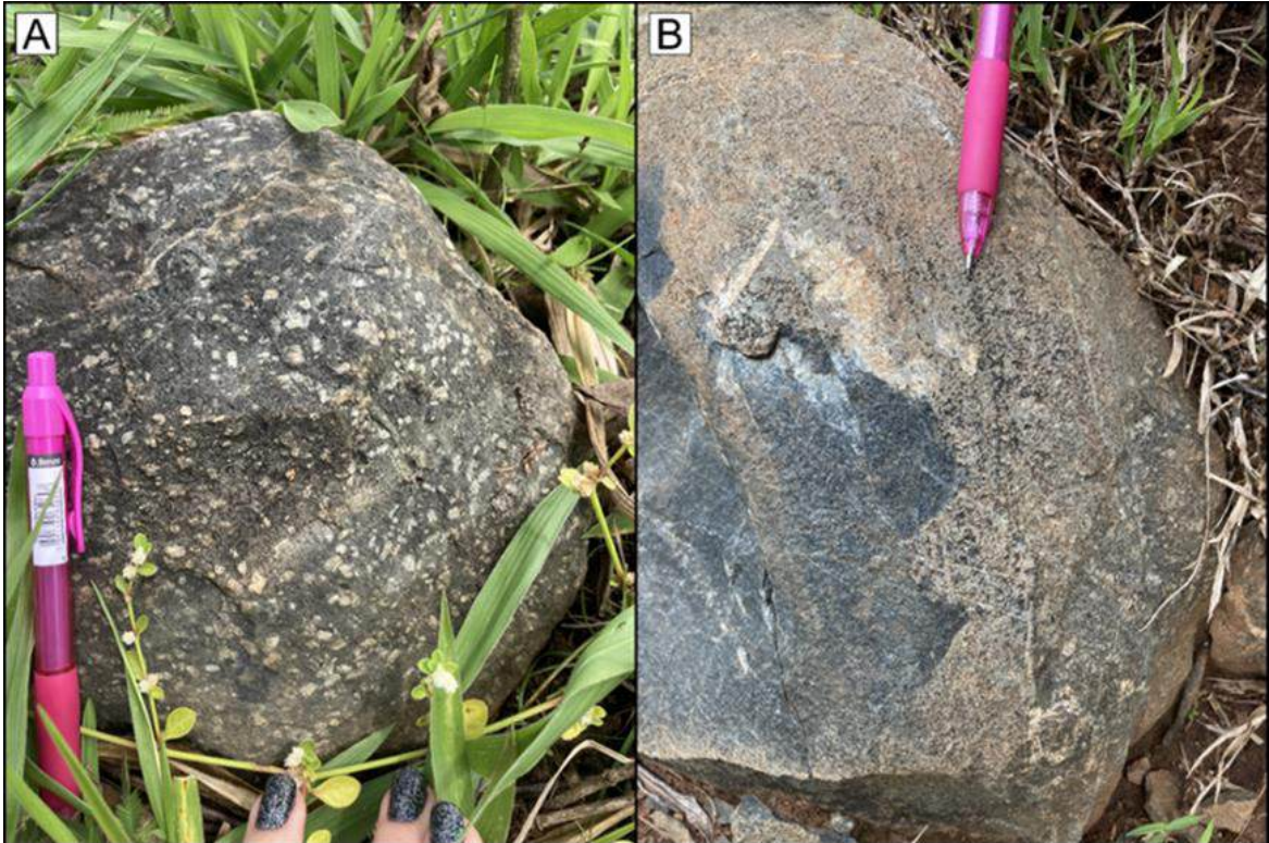
Figure 7-4: : Blocks of mafic to intermediate volcanics; (A) Porphyritic andesite with plagioclase phenocrysts in a fine mafic aphanitic matrix; (B) Dacite with phaneritic texture and crosscut by early system of fine quartz veining.
