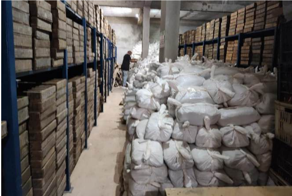
Figure 12-1: Drill core boxes in Canaã dos Carajás core shed. Rejects of crushed samples returned from assay labs are also stored in the core shed Source: GE21, 2024.
