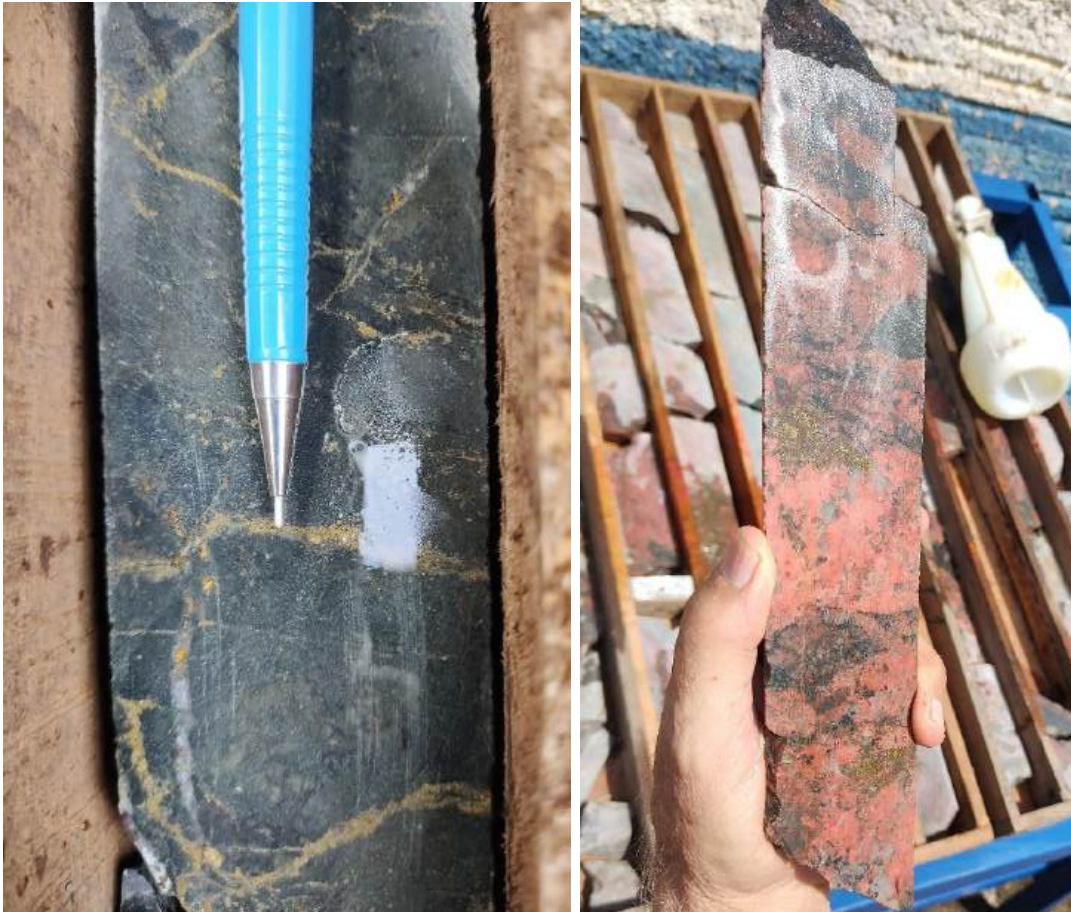
Figure 12-4: Mineralized zones in drill core. High Copper grade zone (left image); and Metasomatite with local occurrence of chalcopyrite (right image).
