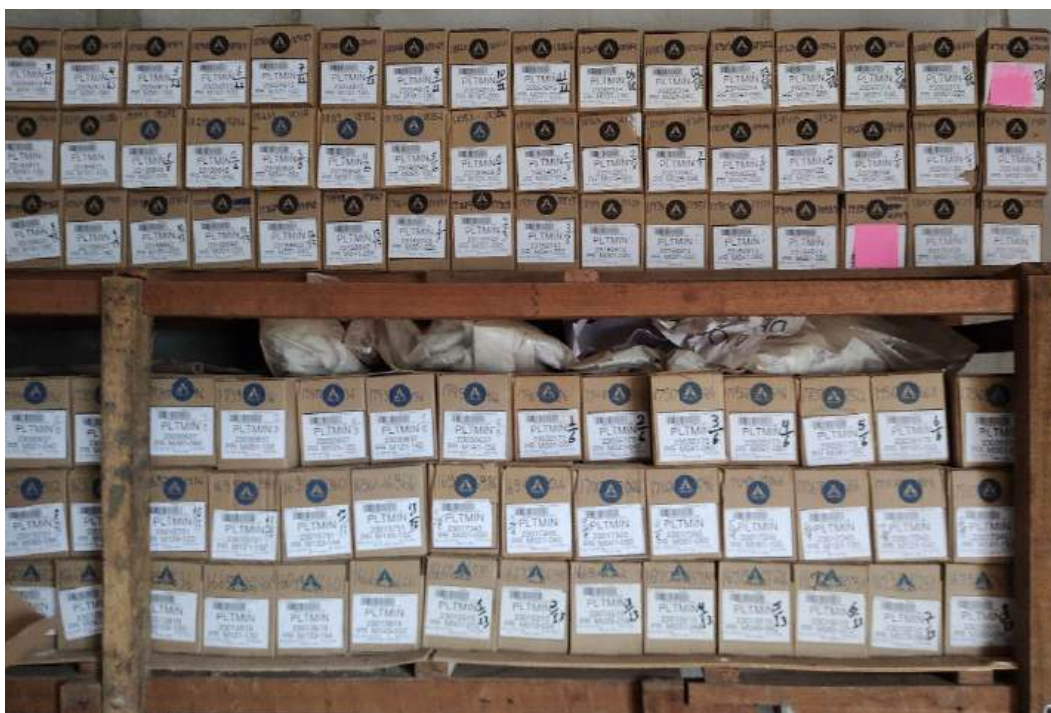
Figure 12-2: Pulverized drillhole samples returned from assay labs stored in the core shed Source: GE21, 2024.
