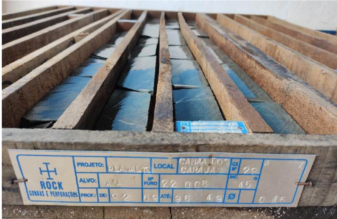
Figure 12-5: Drill core box with aluminum plates with drill core box identification and run markers. Source: GE21, 2024.
