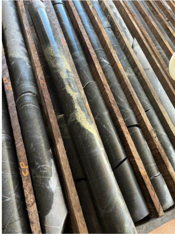
Figure 7-6: Example of drill core with coarse chalcopyrite veining in the volcanics. Source: Planalto Mineração, 2023.
