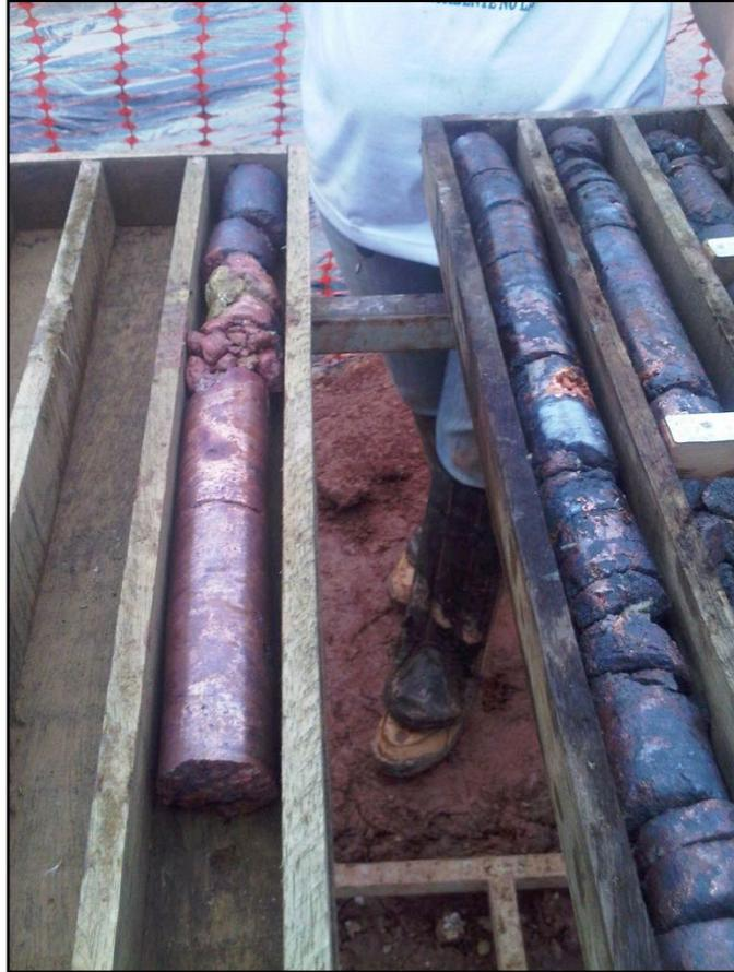
Photo 5 - Detail of high-grade copper mineralization, showing a massive and thick horizon of native copper associated with chalcocite and cuprite in DDH FD-03 (125 m deep).
