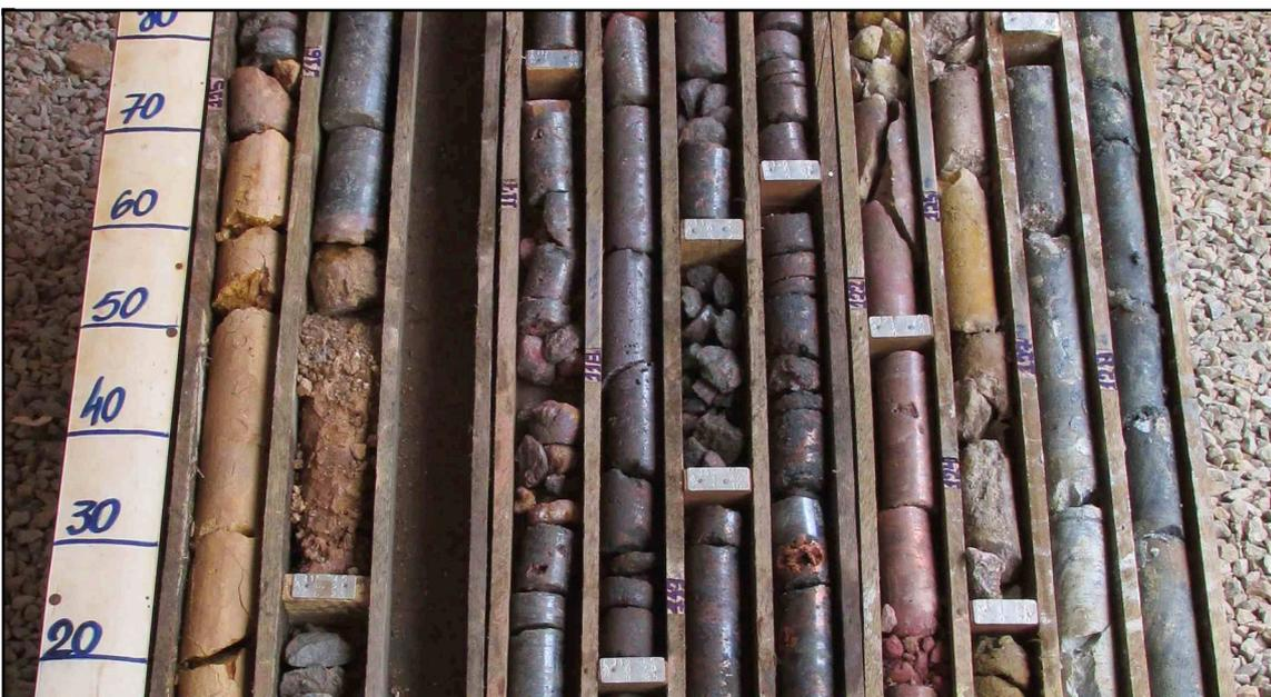
Photo 4 - High-grade copper mineralization in drill cores from DDH FD-03 (110 to 130 m deep), which includes chalcocite, chalcopyrite and native copper. Scale in centimeters.
