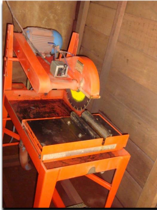
Photo 10 – Drill core cutting equipment.
