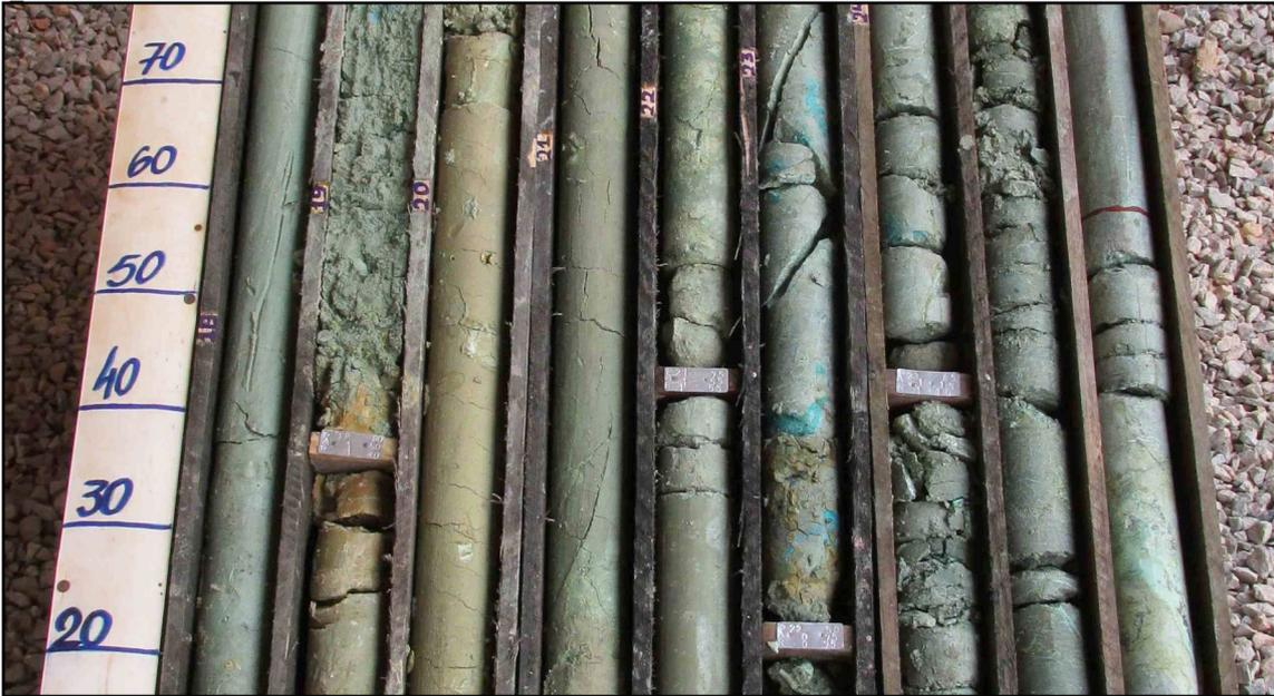
Photo 3 - Oxidized copper mineralization in drill cores, mainly composed of malachite. Cores from DDH FD-03 (0 to 30 m deep). Scale in centimeters.
