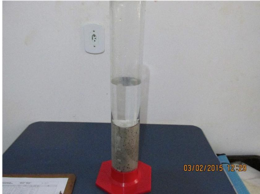
Photo 15 - Measuring the volume of displaced water.
