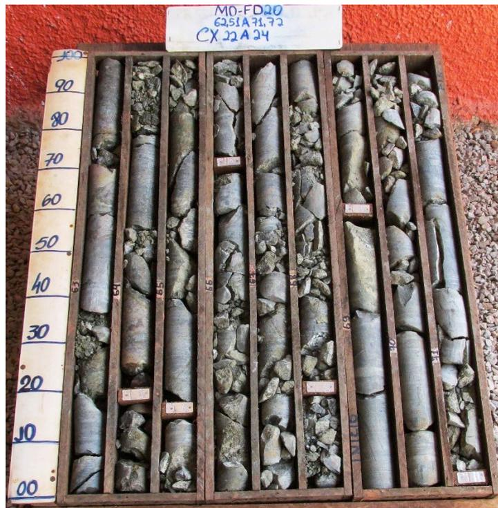
Photo 9 – Example of photographic recording of diamond drill cores of the Osmar Target.
